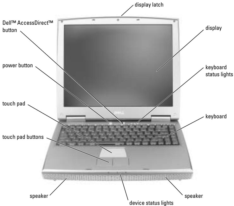
**DISPLAY LATCH** — Keeps the display closed.
