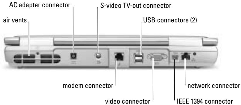
**AIR VENTS** — The computer uses an internal fan to create airflow through the vents, which prevents the computer from overheating.
