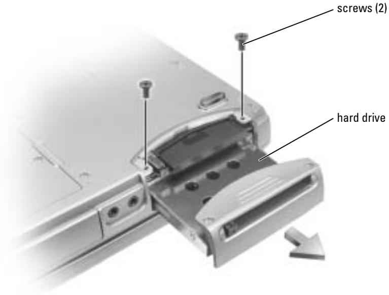
**ⓘ NOTICE:** When the hard drive is not in the computer, store it in protective antistatic packaging. See "Protecting Against Electrostatic Discharge" in the *Product Information Guide*.
